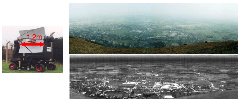
Figure 10. (left) MITRE passive mm-wave imager; (right upper) optical image from Malvern Hills; (right lower) equivalent passive mm-wave image (courtesy of QinetiQ).
