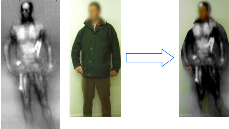
Figure 12. Image fusion and detection (image courtesy Farran Technology 94GHz scanning system and ERA Technology).
