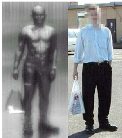
Figure 11. (left) passive mm-wave image of a person with a concealed weapon; (right) corresponding optical image (courtesy of QinetiQ, Malvern).
