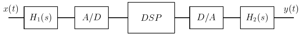
FIGURE 1. Signal chain for the transmitter part of the image communication system. H_1(s) and H_2(s) are anti aliasing and imaging component removal filters, A/D and D/A are the conversion circuits, and DSP is the digital processing unit.
