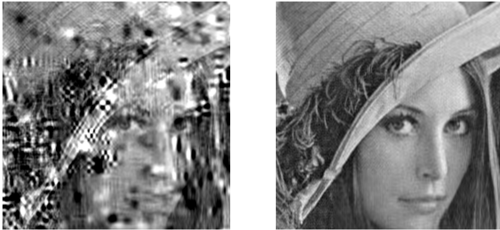
FIGURE 14. Decoded images. Left: random mappings at CSNR=35 dB, right: proposed system at CSNR=20 dB.
