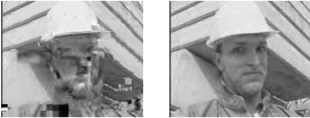
FIGURE 18. Left: Reference system, frame no. 200, CSNR = 17.0 dB. Right: Proposed system, frame no. 200, CSNR = 17.0 dB.
