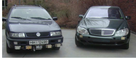
Figure 6. Two experimental cars equipped with 77GHz radar sensors.
